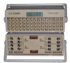
This computerized precision comparator is intended for precise reproduction of the units of complex impedance, and transfer of the value of a unit in the range of measurement, and also for the measurement of capacity (C), inductance (L), resistance (R), the loss tangent (tg $\delta$ ), the phase tangent (tg $\phi$ ), the time constant in the process of metrological works on certification and calibration of the units of complex impedance and also for precise measurement of these parameters.
